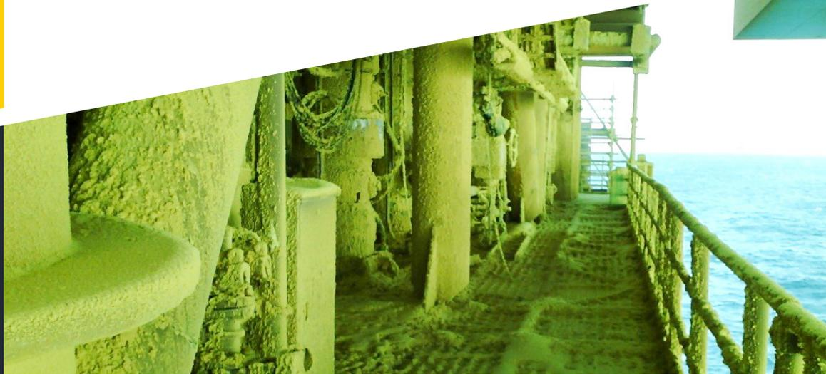
Wild Well successfully deployed a “Floating Mud Cap Well Control” technique to assist in stabilizing and maintaining control during a well control event aboard a floating vessel drilling a deepwater well in the Gulf of Mexico.
